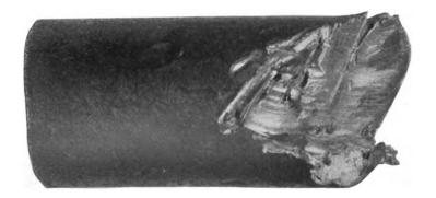
The bolt shown above was cut off by a Disston Spiral Tooth Cut-off Saw in the plant of the Copalis Lumber Co., at Carlisle, Washington. The bolt is one and a half inches in diameter and the cut was diagonal but neither the saw nor teeth were injured in any way. After merely resharpening, the work was resumed. It takes pretty good steel to withstand such unavoidable abuse.
