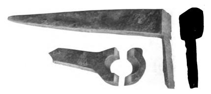
THE gate hinge shown above was embedded in a walnut log which was being cut in the Hoosier Veneer Co., of Indianapolis, Ind. It was struck by a Disston band saw with the result above illustrated. It is of course not an uncommon thing to strike metal in making a cut but the peculiar part of this cut is its absolute symetry. It could hardly have been cut more squarely along the center if it had been measured.
